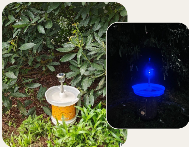
Figure 21: (a) This solar light trap has holders at the base for pheromone lures to support enhanced trapping, as well as a water trap to catch the insects. (b) At night, it emits black light that attracts many insects.
